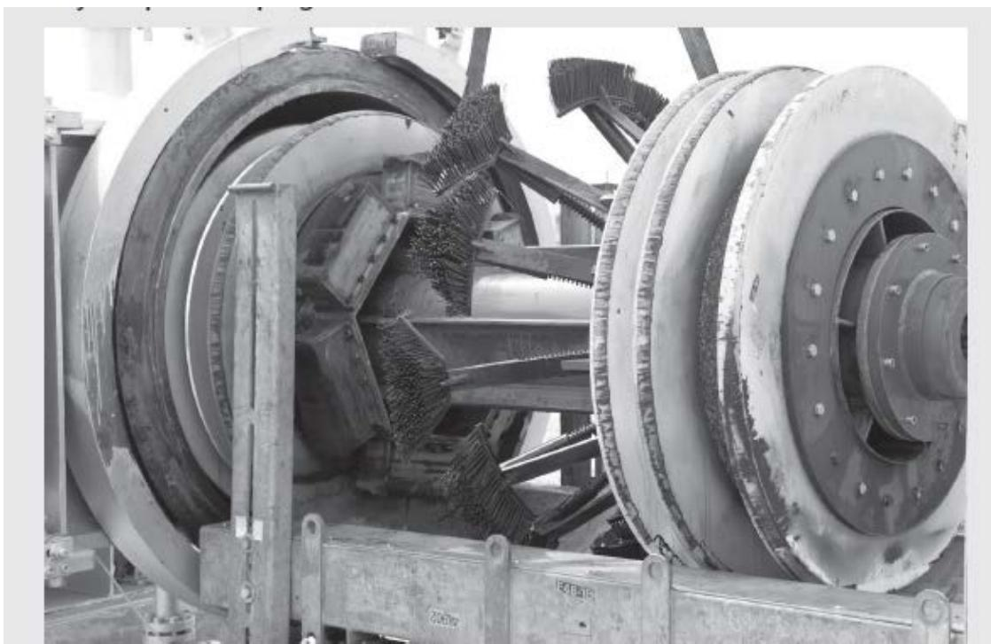
**Figure 12.3.** © Abdelmajidfahim | Dreamstime.com, Pipeline Pig Cleaner Photo
